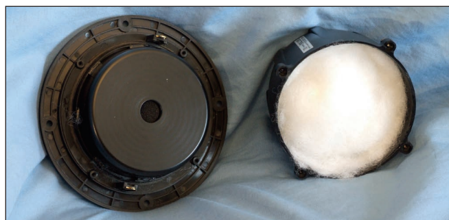
Photo 2: The 75-1558SH's motor system consists of large neodymium (neo) slug magnet with a low carbon content steel return cup with a black emissive coating.
